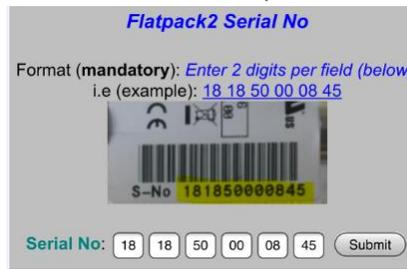
Once Serial No entered, press Submit button. Simple confirmation page will appear, informing that Serial is entered and accepted. At this stage Flatpack2 Control should establish connectivity with rectifier (it may take up to 5-10 seconds) and monitoring data should appear on TFT display:
