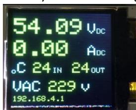
Please note that Load (A<sub>DC</sub> or DC Amperes) will appear only when rectifier is connected and supplying load to DC application, i.e charger, etc. If there is no load connected, the A<sub>DC</sub> will continue to display zeroes.
